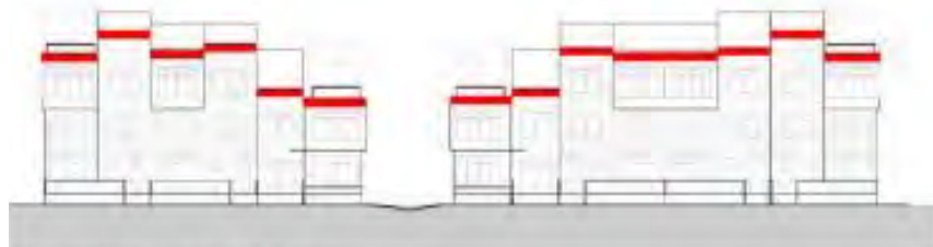
Encouraged - irregular eaveline
